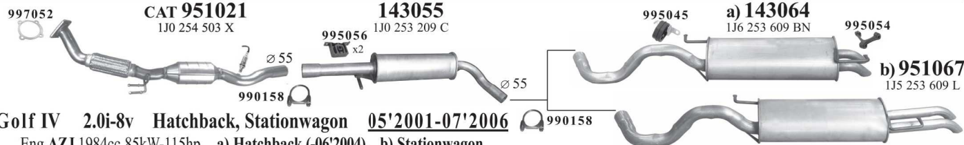
Golf IV 2.0i-8v Hatchback, Stationwagon 05'1998-07'2006 Eng.APK,AQY 1984cc 85kW-115hp a) Hatchback (-06'2004), b) Stationwagon (05'1999-)
