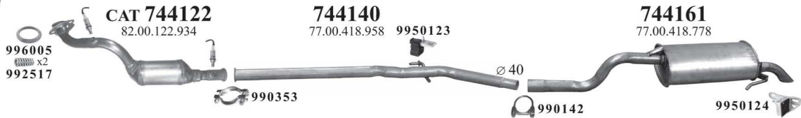
Clio II 1.2i Hatchback 10'2001-11'2011 1.2i-8v: Eng.D7F726, D7F444, D7F746 1149cc 44kW-60hp (-12'2002) 1.2i-16v: Eng.D4F714 1149cc 55kW-75hp (06'2003-), D4F722 1149cc 55kW-75hp (06'2003-) Type BB, CB, SB
