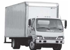
Elf NPR 55-69 2.8D-8v Diesel Truck 10'1993- Eng.4JB1 (OHV) 2771cc 64kW-87hp Type NPR
