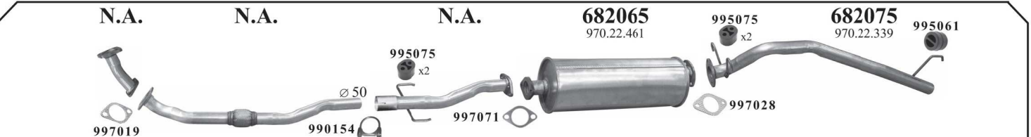
Campo 2.8TD-8v Turbo Diesel Single & Double Cab '1996- Eng.4JB1 2771cc 64kW-87hp Type TFR55 4x2, Type TFS55 4x4
